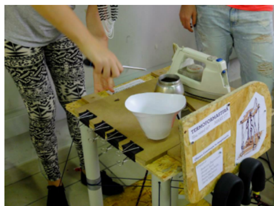
Figure 14. Termoformastira, a domestic thermoforming machine. ( https://vimeo.com/95498670 )
